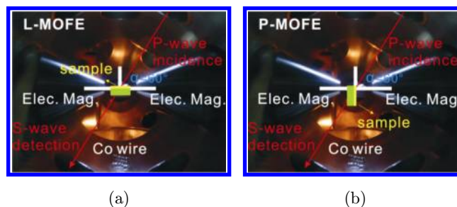
Fig. 1. MOFE technique performed in a UHV system. The Faraday rotation was measured through the detection of transmitted s -polarized light intensity and the rotation of a precise analyzer by the incidence of p -polarized light. Figures 1(a) and 1(b) correspond to the longitudinal MOFE (in-plane field) and polar MOFE (out-of-plane field), respectively.
