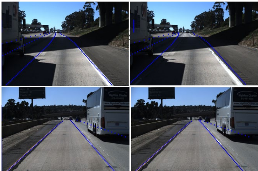
Figure 3. Each row represent the condition on the road, which are lane marks cover by shadow and being blocked by vehicles. The predicted results and ground truth are in the first and second column, respectively.
