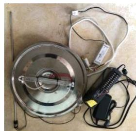
(b) tank lid with a UVC lamp and a temperature sensor mounted
